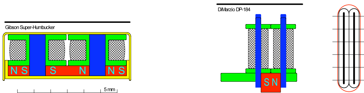
Fig. 5.2.3: Gibson 'Super'-Humbucker [acc. to Lemme] with 3 magnets, und DiMarzio-Humbucker with two metal blades. The Super-Humbucker installed in the L6-S had coaxial coils, however [Billlawrence.com].
